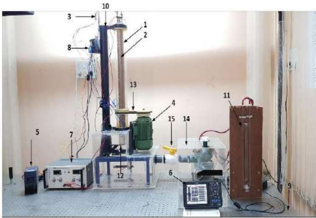
1. Rotating Outer Cylinder, 2. Heated Inner Cylinder, 3. Thermocouple wires, 4. Three Phase AC motor, 5. Variable Frequency drive, 6. Data Acquisition System (Receiver), 7. DC Power Supply, 8. Data Acquisition System (wireless unit), 9. Optical Bench, 10. Frame, 11. U- Tube Manometer, 12. Inner Cylinder Support, 13. Belt, 14. Plenum, 15. Flow control valve
