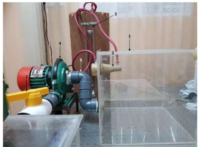
1. Suction plenum, 2. Nozzle, 3. U – tube manometer, 4. Centrifugal blower, 5. Blower inlet, 6. Blower outlet, 7. Flow control valve
